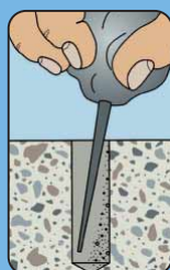
Clean drilled hole
