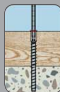
The screw anchor is correctly set when the marking [setting tool] is flush with the surface
