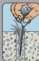
Clean drilled hole
