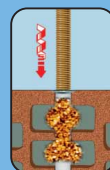
Insert the anchor rod or threaded sleeve into the mortar while slowly turning. Note setting time.
