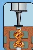
Insert the application tube all the way into the perforated sleeve and fill completely while lifting out in even strokes.
