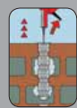
Completely fill with composite mortar from end of sieve sleeve (see enclosed leaflet)
