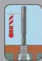
Press in anchoring element up to bottom of sleeve while turning slightly
