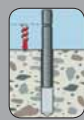
Press in anchoring element up to drill hole base while turning slightly
