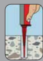
Fill with composite mortar starting from drill hole base (see enclosed leaflet)
