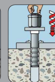
Press in anchor rod up to drill hole base while turning slightly
