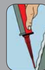
Before use, press out approx. 10 cm bead. Do not use this initial mortar!
