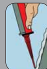
Before use, press out approx. 10 cm bead. Do not use this initial mortar!
