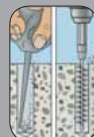
Clean drill hole (blow out 2x, brush out mechanically 2x, blow out 2x), with M16 and larger, blow out with compressed air (compressed-air nozzle).
