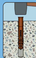
Screw the special screw eye into the sleeve
