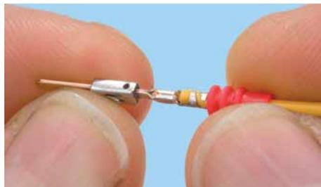
**Slide individual wire seal onto end of wire offset by 180°.\***
