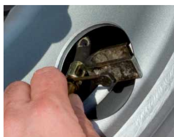
Hose valve extension rubbed through
