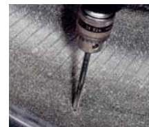
2. Measure the damaged area in order to choose the body. Drill out the cutting channel from the inside out.
