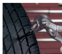
7. Pull the probe out from the outside until the disc of the repair body is lying flat on the inside of the tyre.
