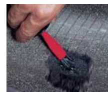
5. Add a drop of solution to the cutting channel. Spread the solution on the roughened surface. Let the solution dry for 5 minutes.
