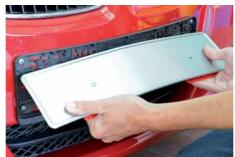
The combination is now pushed from below (or from above if appropriate) into the closed license plate holder. The license plate is then pressed upward – while simultaneously pressing against the vehicle – (or downward if appropriate) with your fingers until the quick-action license plate holder clip engages below (or above).
