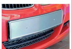
► Please ensure that the top and bottom clip closures engage securely behind a retaining tab or frame of the license plate holder. If this is not ensured, the clip may not be used!
