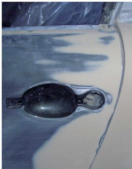
**Knifing filler for filling and leveling deep uneven areas and scratches.**
