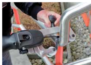
Disks as a contact surface for guiding the belt
