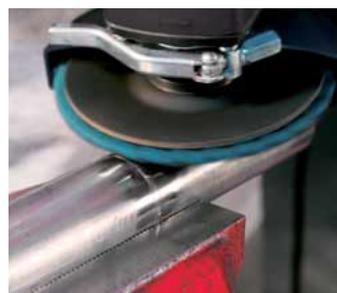
Grinding welding seams and removing thermal blue discolorations
