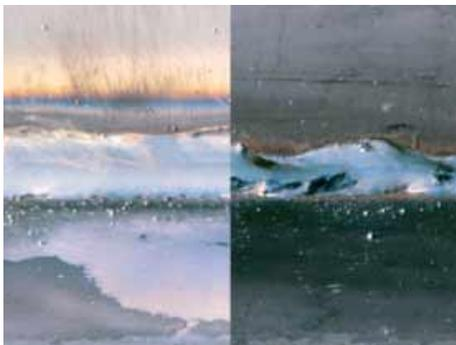
Surfaces descaled before welding result in cleaner weld seams (see Fig. on left).
