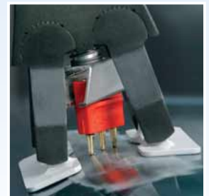
The pulling axis is freely rotatable around 360°.
