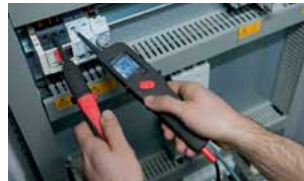
DC voltage test
