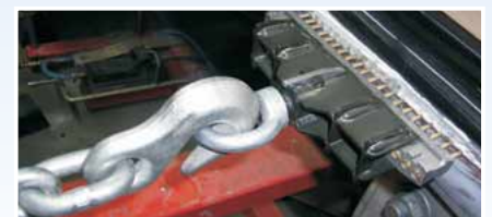
Pulling cross piece with pulling ring on the chain of a car bench.
