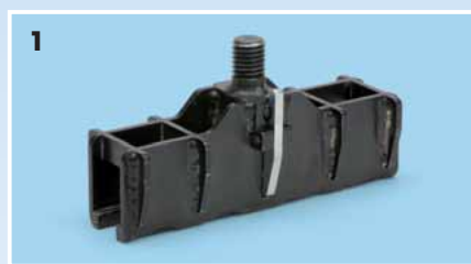
Undo the deformation with a slide hammer or a pulling tool.
