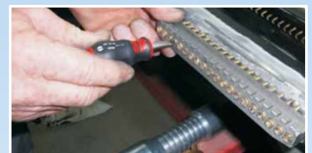
Using Screwdriver 0613 251 065, turn the pulling electrodes 90°. You're done!
