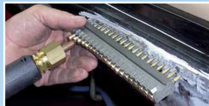
Place Copper Electrode 0691 500 178 on the countersunk head and weld it on.
