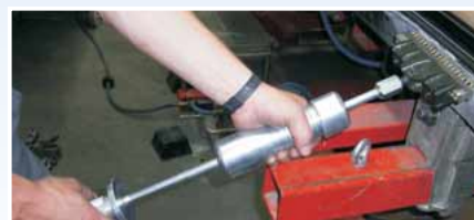
Pulling cross piece with slide hammer for quick dent removal.
