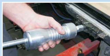
Undo the deformation with a slide hammer or a pulling tool.
