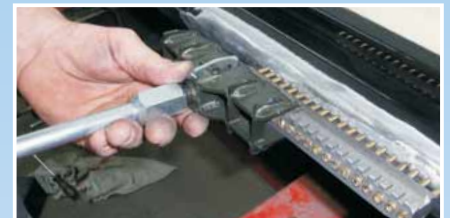
Guide pulling cross piece into the pulling block and engage the catch at the desired position.
