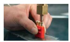
Place the copper electrode on the countersunk head and weld.
