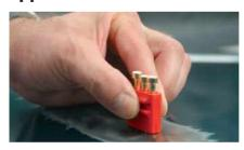
Place tips of electrodes on the metal sheet and push down the puller block.
