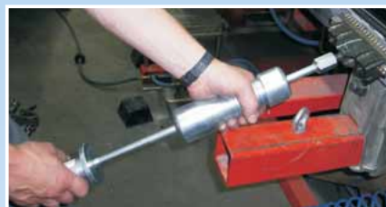
Pulling cross piece with slide hammer for quick dent removal.
