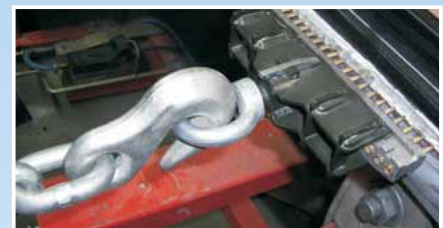
Pulling cross piece with pulling ring on the chain of a car bench or dozer
