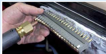
Place copper electrode on the countersunk head and weld it on.
