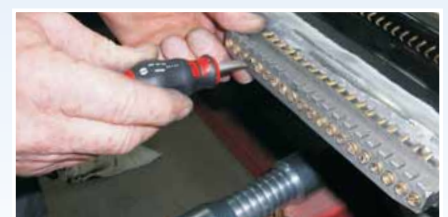
Using the screwdriver, turn the pulling electrodes 90°. You're done!
