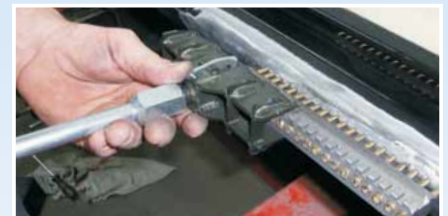
Guide pulling cross piece into the pulling block and engage the catch at the desired position.
