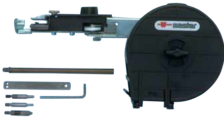
Adapter for ASSY®mat 80 For screws 3.5 x 35 - 4.2 x 50 mm. Art. No. 0702 164 3
