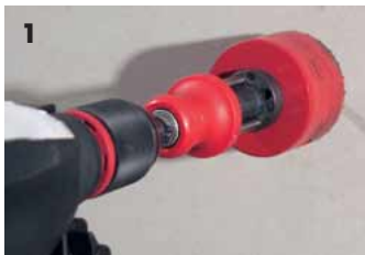
1 Drilling of hollow-wall device sockets, halogen lamps etc., in gypsum plasterboard, for example.
