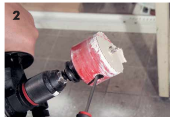
2 The conventional method: Ejecting the cut-out material is very difficult and can only be done with an additional tool.
