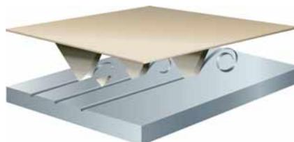
Precision-formed uniform abrasive grits have an even distribution and uniform alignment. This results in maximum removal performance and a perfect surface finish.
