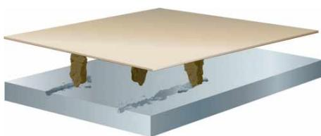
Conventional ceramic grits come in different shapes and sizes and have an uneven distribution. The grits "plow" the surface and heat is produced.
