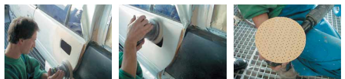
Sanding of knifing filler with Useit® Superpad P vehicle, 100 grain
