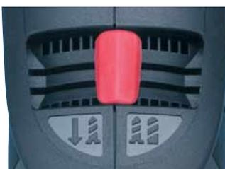
Clockwise/counterclockwise switch on the top of the housing ensures maximum torque in both rotation directions via optimum positioning of the carbon brushes and extends the service life of the carbons considerably.
