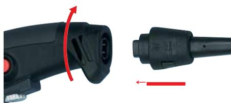
Changeable connection cable: Turn cable plug to the left and remove cable. Insert new cable and lock by turning to right.
