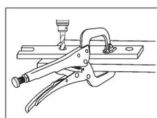
**High, wide clamping arm with movable clamping jaws.**
