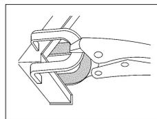
**U-shaped gripping jaws, upper gripping jaw is angled downward 90°.**
