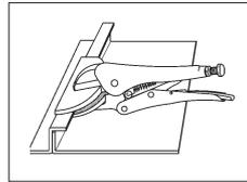
**Wide, flat clamping jaws for especially high surface pressure.**
