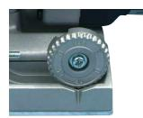
The cutting depth can be adjusted with the adjusting wheel to sizes 0, 10, 20, Simplex, Duplex and Max.
