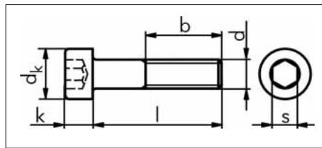
"DIN 912 was withdrawn and replaced by the international standard ISO 4762".
