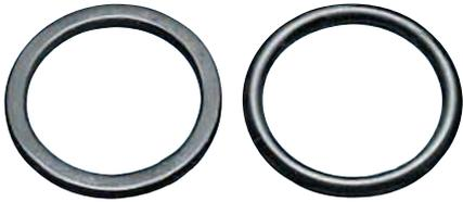
Generally, all rings in accordance with DIN 7603 are flat seals on resting surfaces. They are used for sealing on static pipe screw joints. The material from which the sealing rings should be made depends mainly on the media found in the pipeline.
